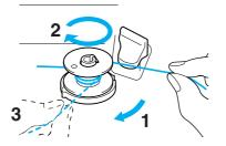
Pass the end of the thread through the guide slit in the bobbin winder seat, and then pull the thread to the right to cut it with the cutter.
